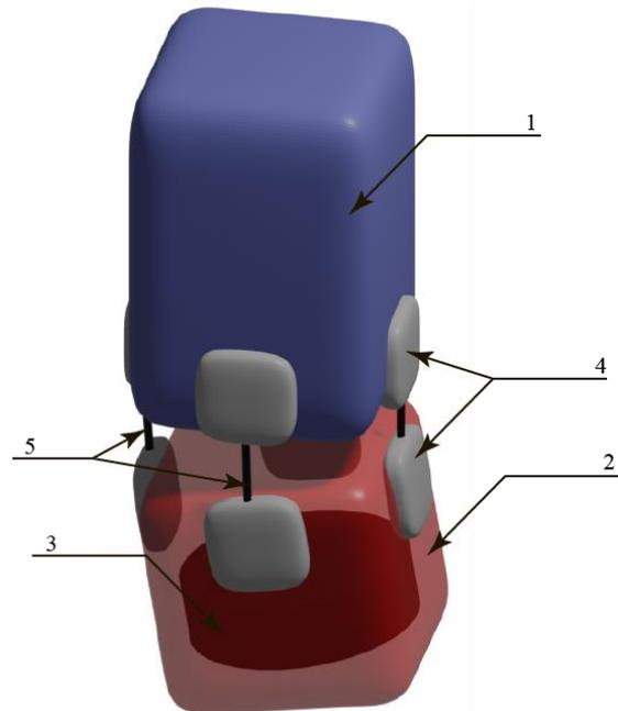
1 - carrier body, 2 - movable module, 3 - internal rotor, 4 - flexible rod control system, 5 - flexible rods.
